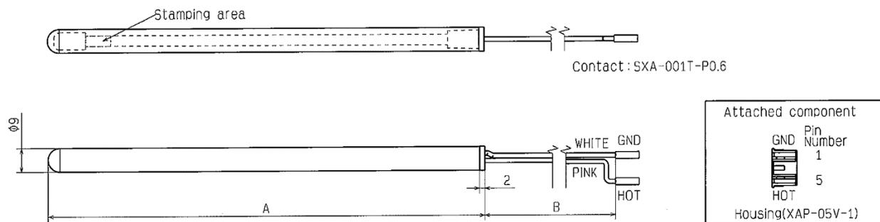
\* The housing that connect with the edges of wire harnesses, will be attached as a another part of this assembly.
