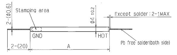
The high voltage side is recommended to be connected with The side without marking.
