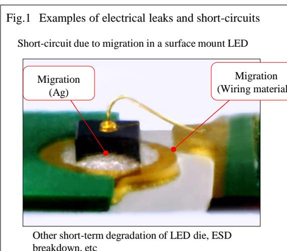
Electrical leaks and short-circuits are caused either by faults or degradation in the semiconducting properties of the LED die, or by electrochemical changes in the materials used.
