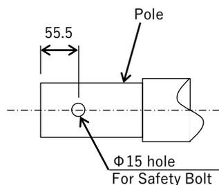
**Installation procedure****1. Open cover**
