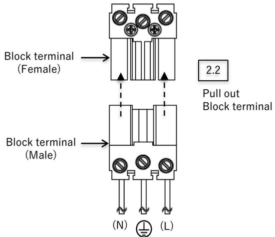
2.3 Connect AC line cable to Terminal Block (Female) by using "-" driver
