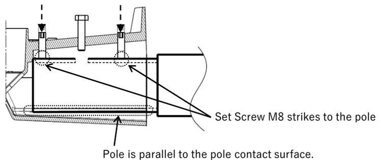
**3. Install Hexagonal Bolt M8 for safety to  $\phi 15$  hole of housing.**
