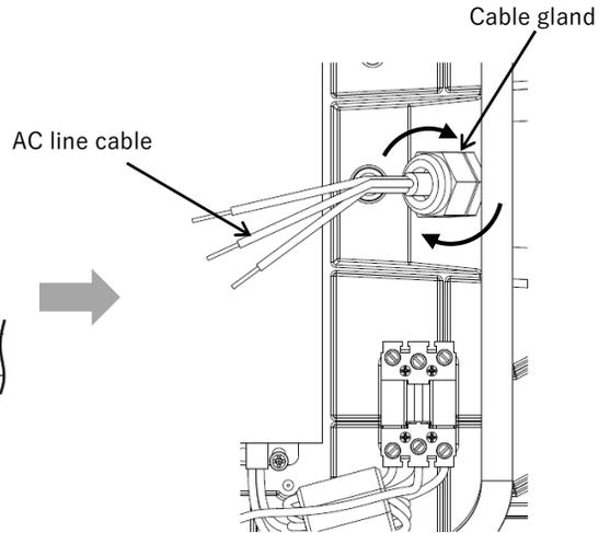
2. Connect wire of AC line cable to Terminal Block (Female)
