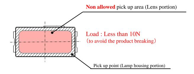
Please adjust the load, the pick up point, the nozzle diameter and etc. before mounting because the over load can cause the breakage of the lamp housing.
